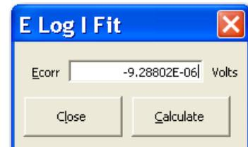
You can run a Polarization Resistance fit on this Potentiodynamic data, if the axes of current are changed to the linear scale. Generally we suggest running a separate experiment on a new sample of the same material because of the more-polarizing, more-destructive nature of the Potentiodynamic experiment.
